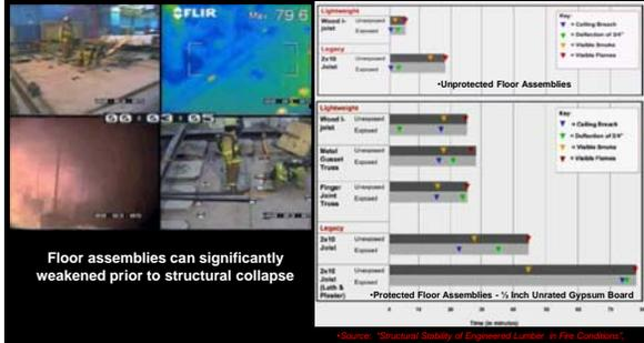
Floor assemblies can significantly weaken prior to structural collapse
