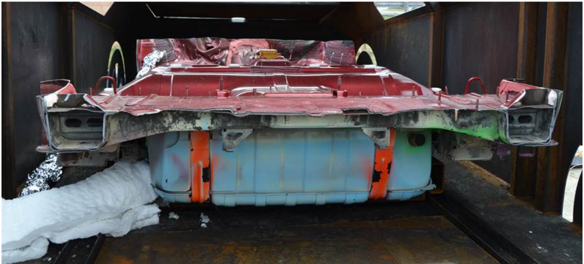
Figure 34 View of Battery B inside the VFT without the floor pan (top) and with the floor pan (bottom); the blue tank at the rear of the battery is the empty gasoline tank for the production vehicle, which blocks direct access to the rear of the battery
