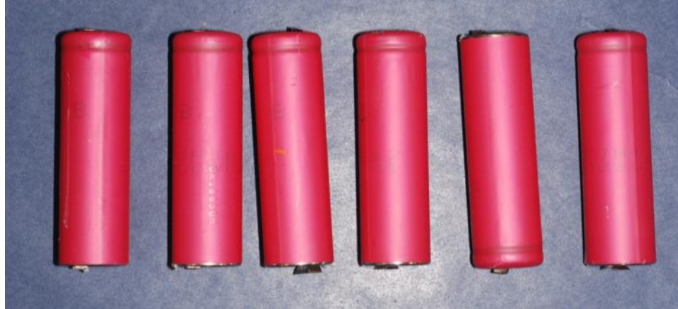
Figure 3 Example of 18650 cylindrical cells (these are the most common consumer electronics Li-ion cell form factor)
