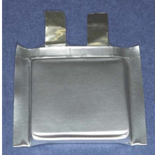
Figure 5 Example of a soft-pouch polymer cell
