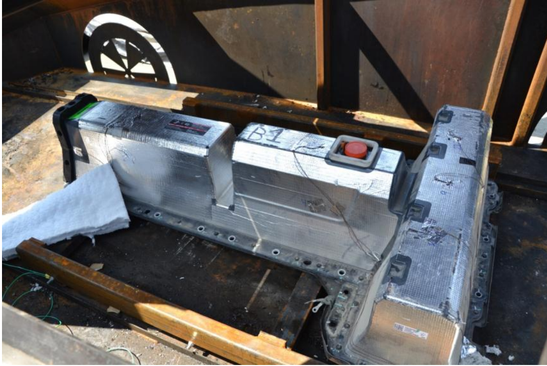
Figure 27 Battery B positioned on the carriage above the burners inside the VFT; burners located in the center test position
