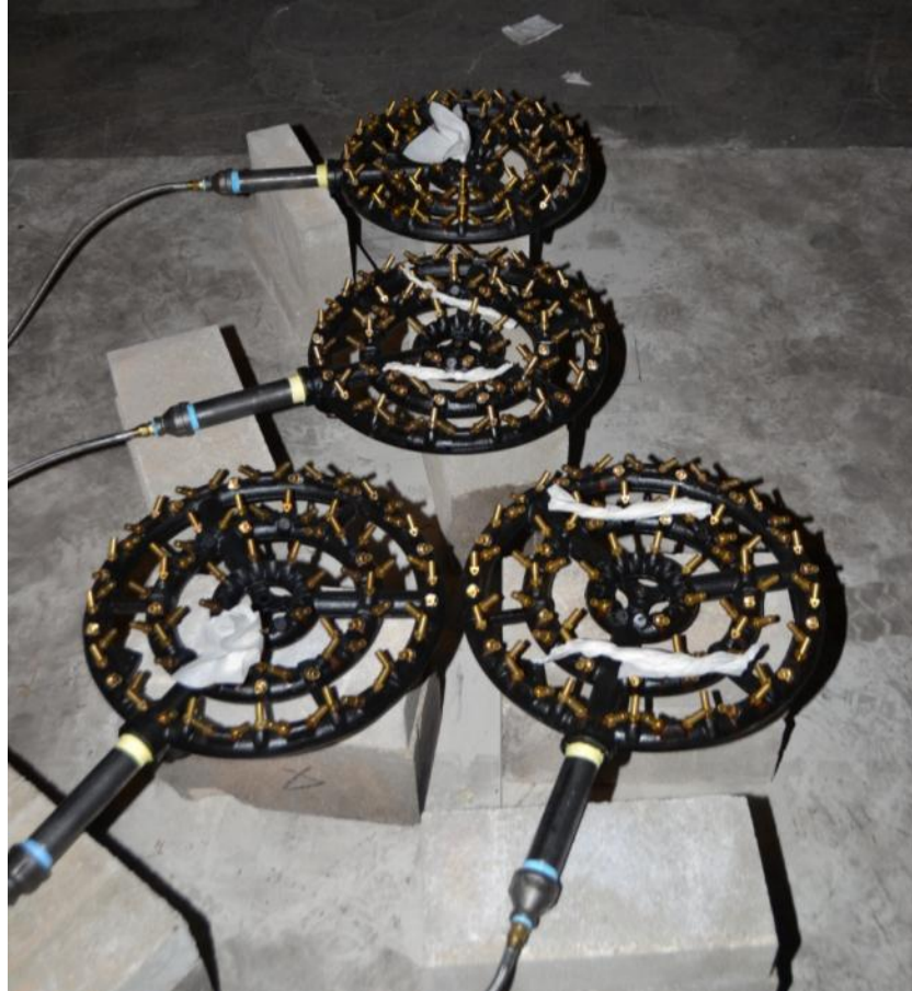
Figure 15 T-shaped burner arrangement comprised of four burners
