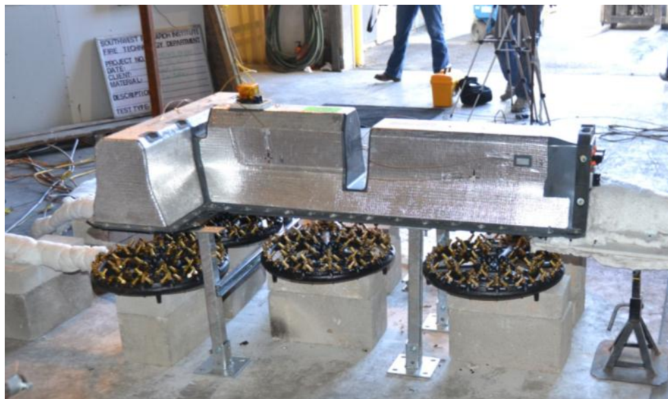
Figure 15 T-shaped burner arrangement comprised of four burners
