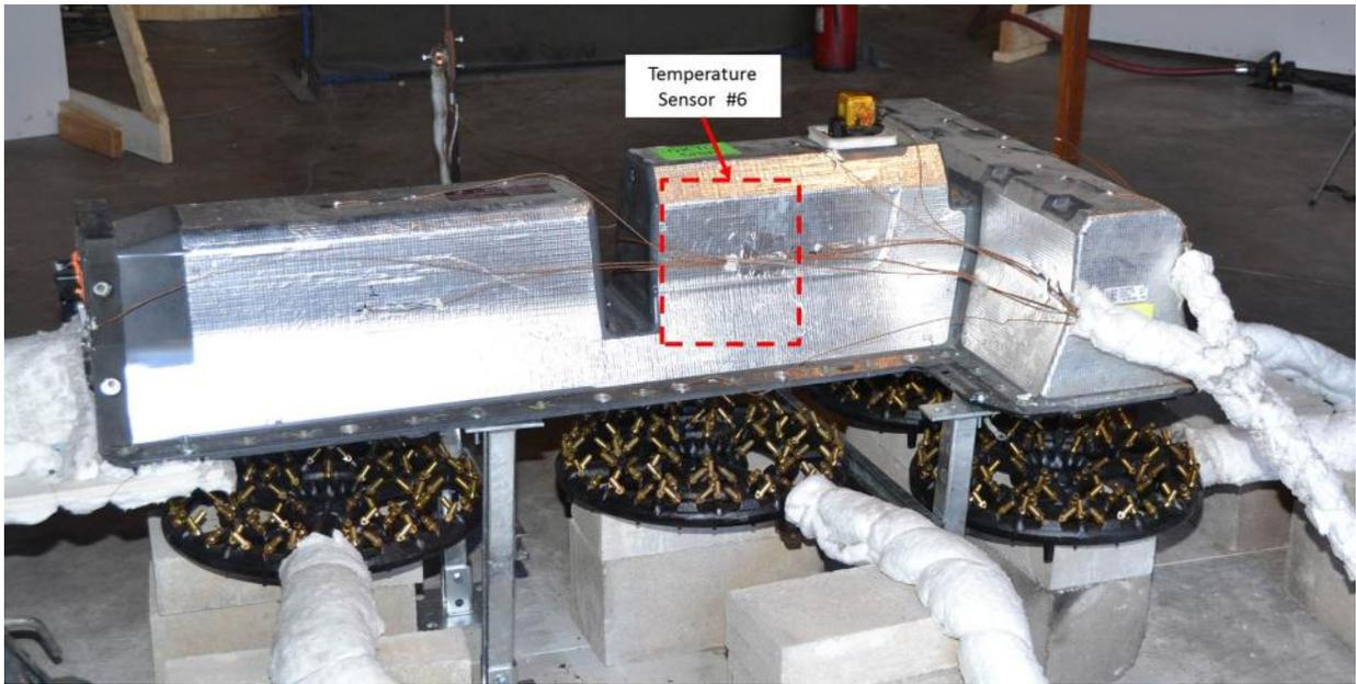
Figure 85 Location of temperature Sensor #6 within Battery B2
