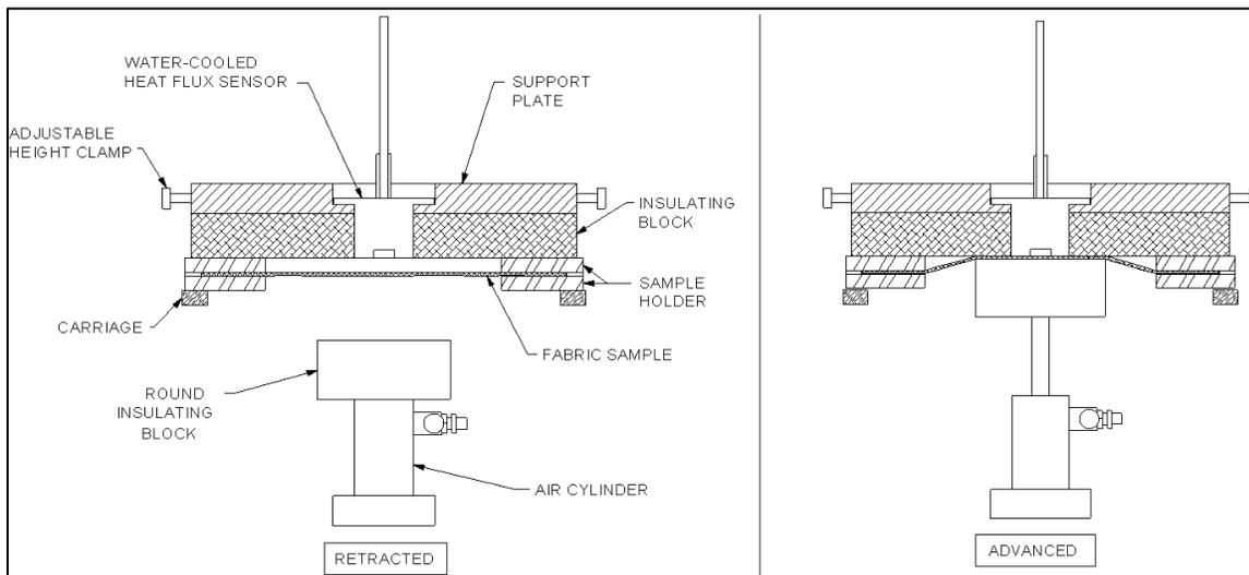
Figure 9. Compressor assembly
