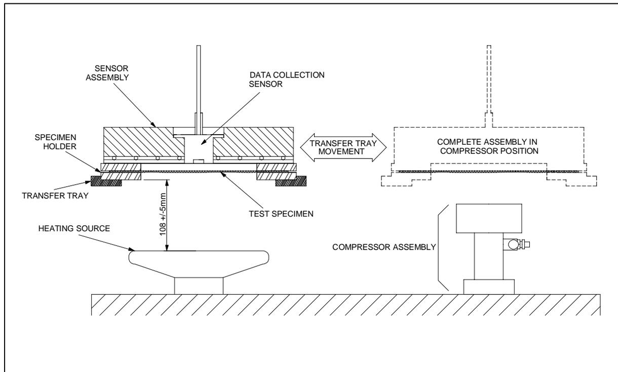
Figure 6. Stored thermal energy test apparatus (top view)
