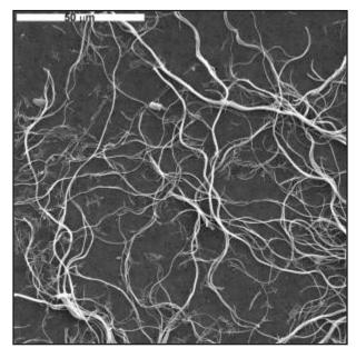
Figure 2-10.1: Chrysotile Asbestos Fibers.
