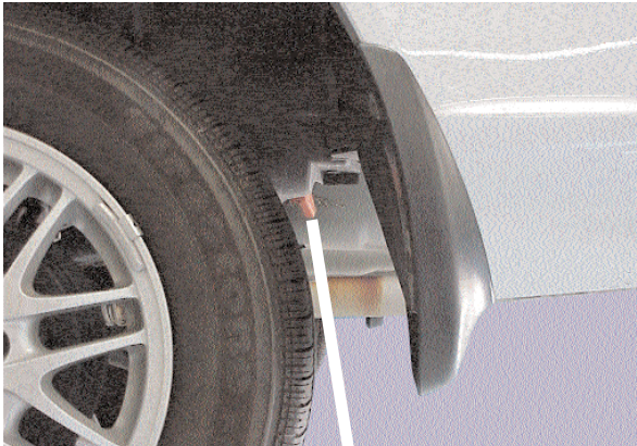
CNG Manual Shutoff Valve
