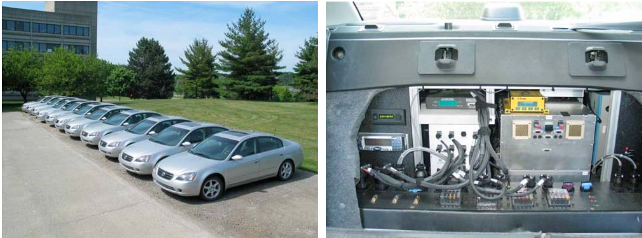
Figure 3. The fleet of instrumented vehicles (2003 Nissan Altima 3.5SE sedans), and a view of the main instrumentation package in the trunk of one of the vehicles.
