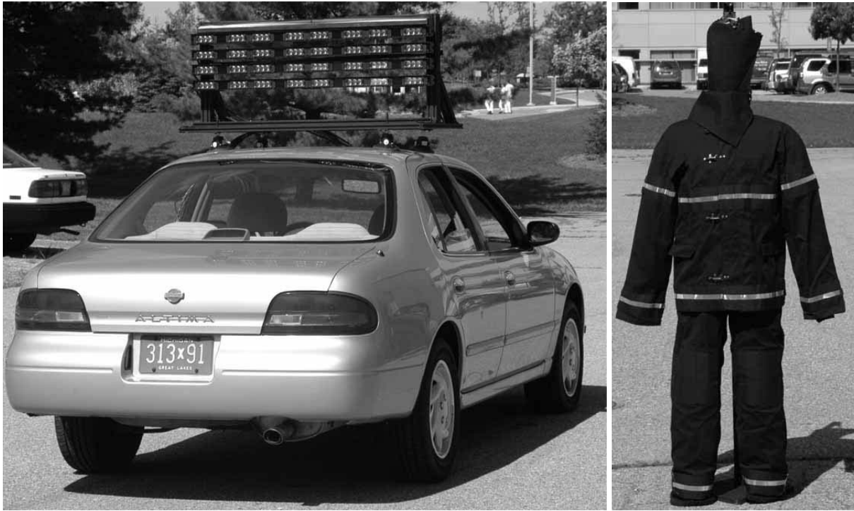
Figure 4. The car that was used as the stationary vehicle, with the experimental warning lamps mounted on its roof, and one of the pedestrian mannequins, showing the retroreflective strips.
