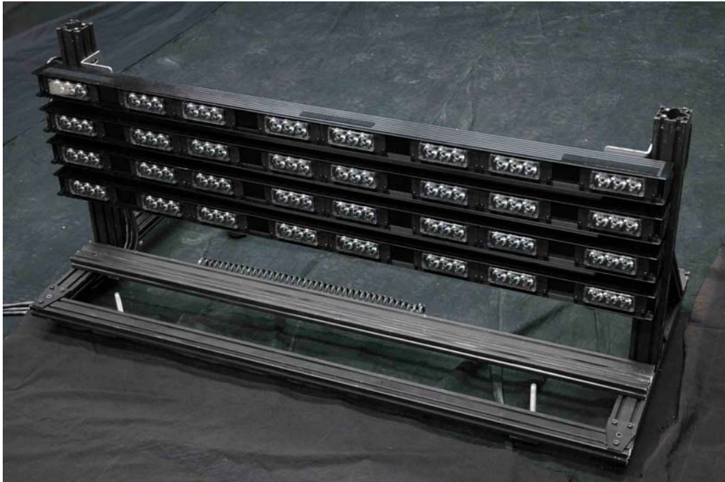
Figure 6. The LED lamp array that was used on top of the parked vehicle.
